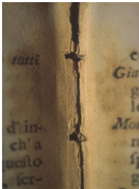
Fig. 15 The effect of humidity and intrinsic acidity on binding of a 1700s book
